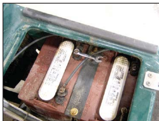
25. Negative Battery Connection
